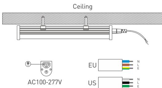
(3). Fixed rotatable clips & fixture with tighten screws.
