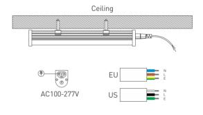
(3). Fixted rotatable clips & fixture with tighten screws.
